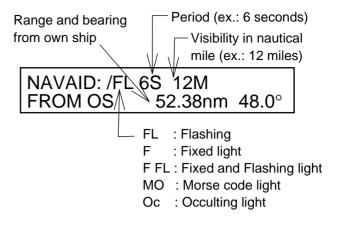
Figure 3-7 Example of buoy, lighthouse data
